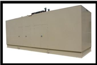
Similar in design to the Weather Proof enclosure, this model offers more sound attenuating foam, and has larger air chambers. Fixed air intake louvers, housed within their own air chamber, along with 1.5" foil coated foam and a bird screen make this enclosure very popular. Expected noise levels for this unit are about 3-4 dB less than the Weather Proof enclosure with foam and scoops. This enclosure design is used on DDC/MTU Power Generation models, which are 250kW and above.
